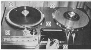
FIG. 6-45. Top view of Ampex magnetic-tape recorder. The various functions of the instrument are controlled by push buttons (1). The capstan is driven by a synchronous motor. The take-up (2) and supply reel (3) are driven by motors so designed as to provide relatively constant torque independent of diameter variations of the reels. The head assembly has a sliding frame, the position of which is controlled by the handle (4) on the rear of the head housing (5). When the gate (6) is closed, the recording medium (7) is given a slight wrap around the pole pieces of each of the three tape heads—the recording (8), the erasing (9), head. With the gate open, the tape can be moved at high speed.
