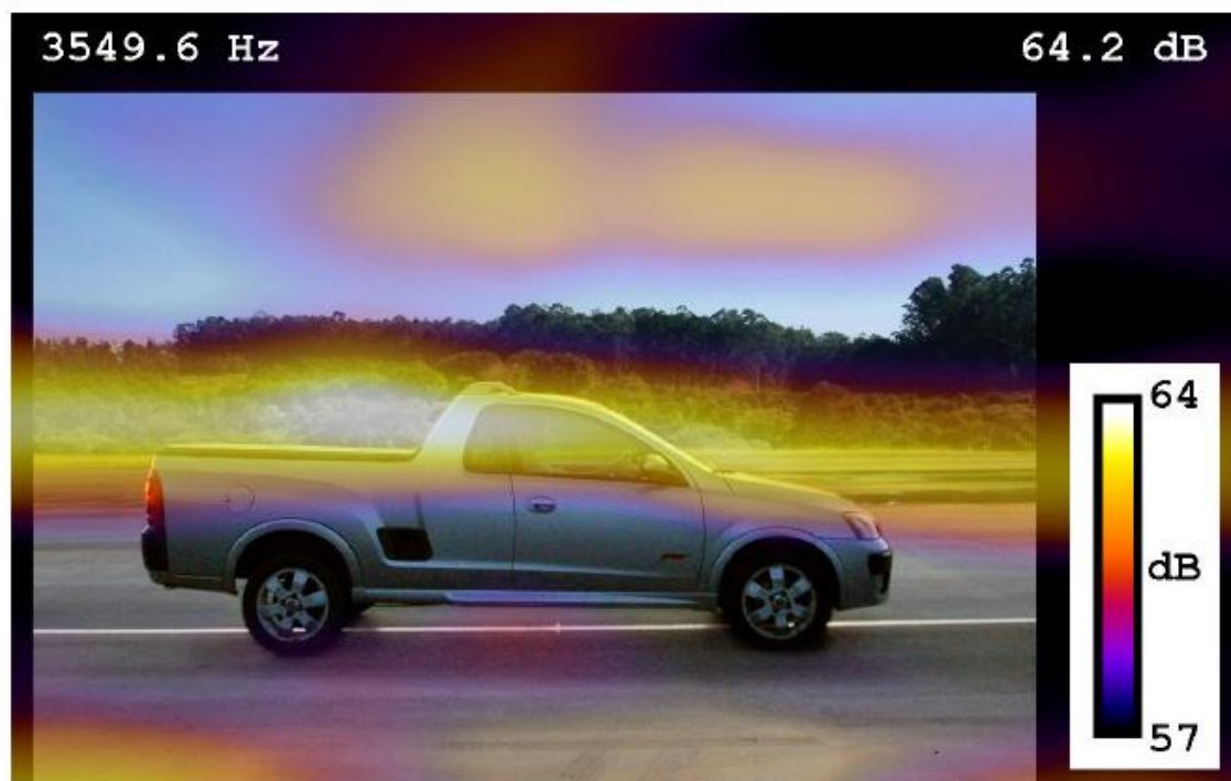
Figure 5: Beamforming data without de-dopplerization.
